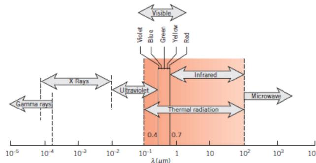
FIGURE 12.3 Spectrum of electromagnetic radiation.
